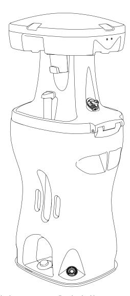
All materials, including resin, pigments and additives used to make the plastic components as well as the plumbing components that come in contact with the fresh water are U.S. FDA food grade compliant.
